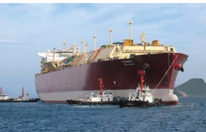
When delivered to Qatar in October, the LNG ship Tenbek will be the world's largest, with a capacity of 216,200 cubic meters.
